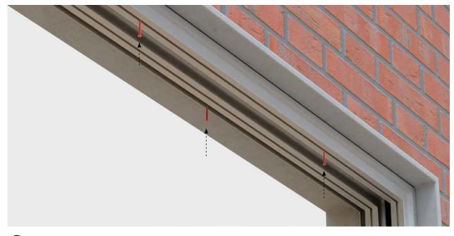
14 Where possible, fixing points should be on both sides of the frame, in a zig-zag pattern.
