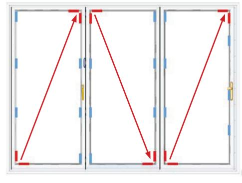
Use 'Toe and Heel' Load Bearing Packers for panel alignment
